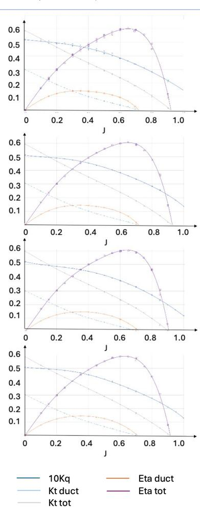
The first part of the experimental activity was conducted last July and August in the large towing tank of CNR-INM (i.e. 470 m long, 13.5 m wide and 6.5 m deep). Tests included open water propeller performance measurements and resistance measurements.
