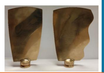
A comprehensive numerical and experimental survey has been conducted from NEWCASTLE UNIVERSITY, CNR, CHALMERS and DST to insight into the propulsive performance and the hydrodynamics of tubercle propellers. NEWCASTLE UNIVERSITY continued openwater testing of its newly designed propeller featuring tubercles, in the Emerson cavitation tunnel (emerson cavitation tunnel).
